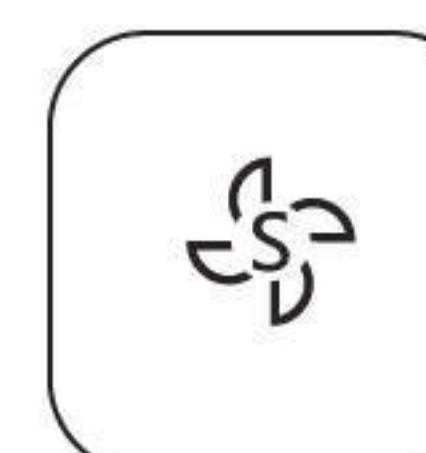
Touch again, the smoke shield will be On, the indicator will flash, and the range hood will run at the transient absorption gear. Touch again, the indicator will be fully lit, and the range hood will run at strong gear. Touch the third time, the indicator will be Off, and the fan will stop running.
